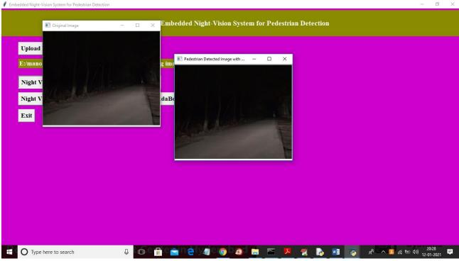
In above screen first image is the original image and second image is the YOLOV2 resultant image and in second image we did not find any bounding box across pedestrian so YOLOV2 unable to detect that pedestrian and now click on 'Night Vision Pedestrian Detection using HAAR + AdaBoost' button to get below result
